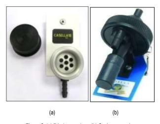
Figure 2: (a) 7-hole sampler; (b) Cyclone sampler
